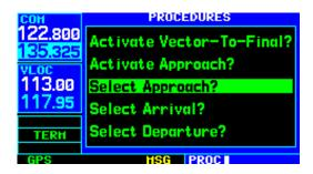
3) A window appears listing the available procedures. Turn the large **right** knob to highlight the desired procedure and press the **ENT** Key.
