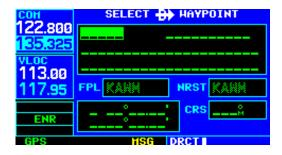
2) Use the small and large **right** knobs to enter the identifier of the desired destination waypoint.
