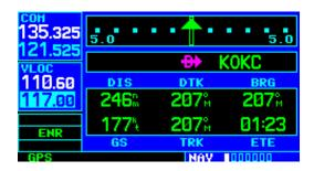
3) Turn the small **left** knob to select the desired kilohertz (kHz) value. For example, the '.80' portion of the frequency '117.80'.
