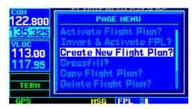
4) A blank Flight Plan Page appears for the first empty storage location. Use the small and large **right** knobs to enter the identifier of the departure waypoint, and press the **ENT** Key.
