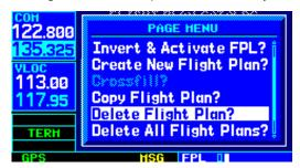
4) With 'Yes?' highlighted, press the **ENT** Key to delete the flight plan.
