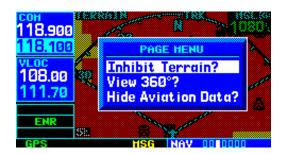
2) Press the **ENT** Key. The 'TER INHB' annunciation is displayed in the TERRAIN annunciator field when TERRAIN is inhibited.
