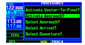
The 'Activate Vector-To-Final?' option allows the pilot to activate the final course segment of the approach. This option assumes the pilot will receive vectors to the FAF and provides guidance to intercept the final course, before reaching the FAF.
