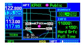
6) To view the other airport information pages, press the small **right** knob to remove the flashing cursor and turn the small **right** knob to select the desired page.
