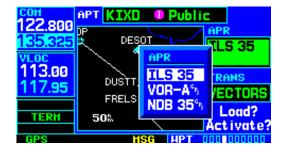
4) A second window appears listing the available transitions. Turn the large **right** knob to highlight the desired transition waypoint and press the **ENT** Key. (The approach 'Vectors' option assumes the pilot will receive vectors to the final course segment of the approach and will provide navigation guidance relative to the final approach course.)
