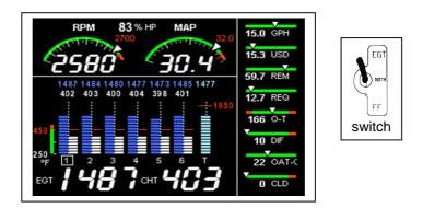
EDM-830 system mounts in a 3.125 inch instrument panel hole in either a portrait or landscape position depending on panel hole location.
